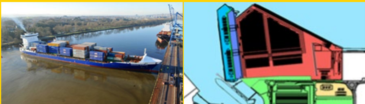
Picture 2: demonstrates the limitations at the existing Lo-Lo facilities in the Tivoli Container Terminal (water depth, width for vessel swinging, landside terminal capacity).
