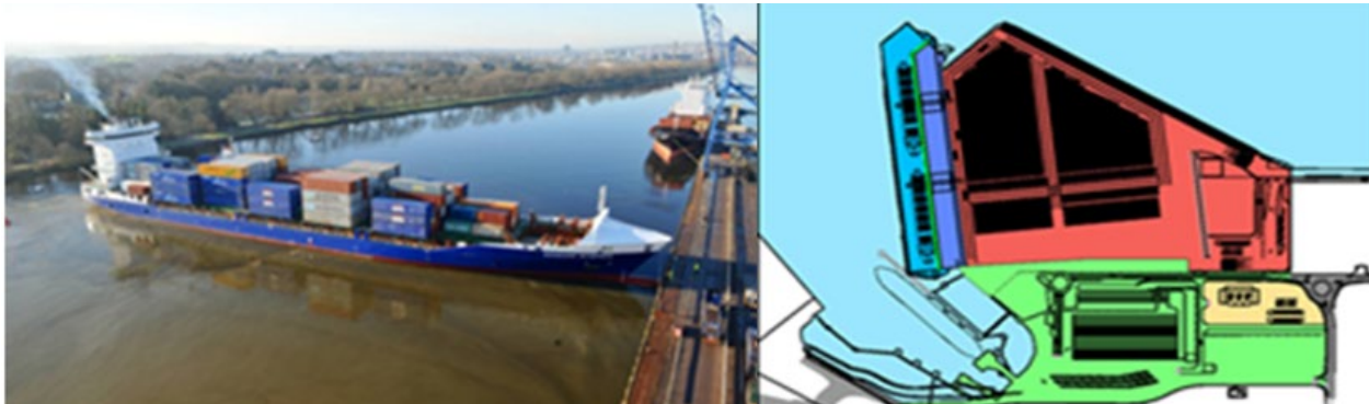
Picture 3: demonstrates the limitations at the existing Lo-Lo facilities in the Tivoli Container Terminal (water depth, width for vessel swinging, landside terminal capacity).
