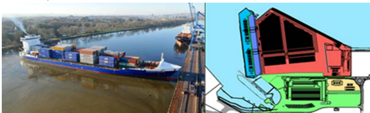
Picture 5: demonstrates the limitations at the Lo-Lo facilities in the Tivoli Container Terminal (water depth, width for vessel swinging, landside terminal capacity).
